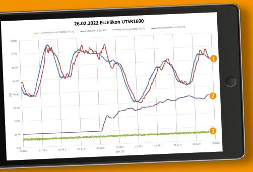
Values reflect fuel change from dry waste wood M 10 to moist forest residue wood M 35.
